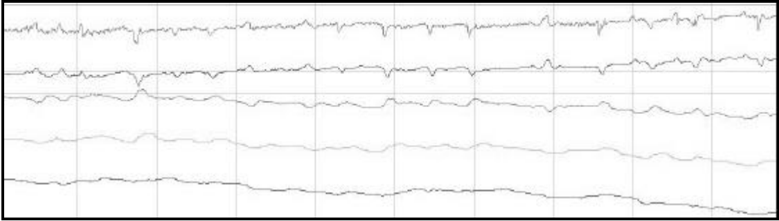
Figure 3: A) Original FHR signal. B, C, D, E) The first principal component of the FHR signal obtained respectively, at sample sizes of 15, 30, 60 and 120 in the input to the MR-PCA network.
