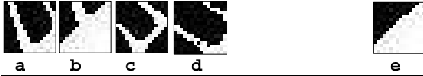
Fig. 6. Some examples of 16x16 searchboxes on identical spot in different test-images. (a-d): test-images with a defect called 'hairs', (e): searchbox on identical spot in the adequate template.
