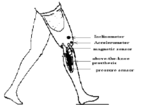
Figure 2: The above-the-knee prosthesis and its sensors
