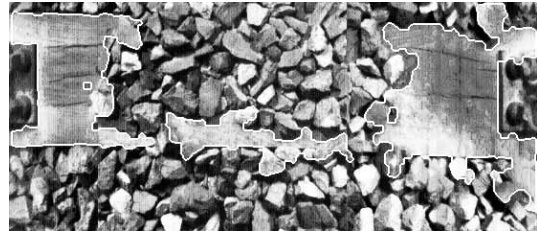
Figure 9: A detected boundary contour of a wooden tie
