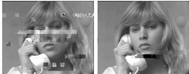
Figure 2. Frame number 84 obtained from the simulation runs for the 2 TS scheme (left: 30 db, right: 38 db)
