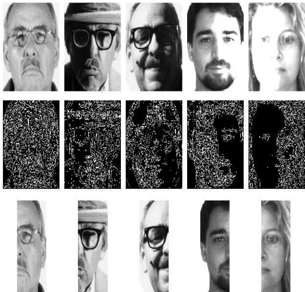
Fig. 2. (a) First row : Test Images (b) Second row : Edge Densities (c) Third row : Picked Half-faces
