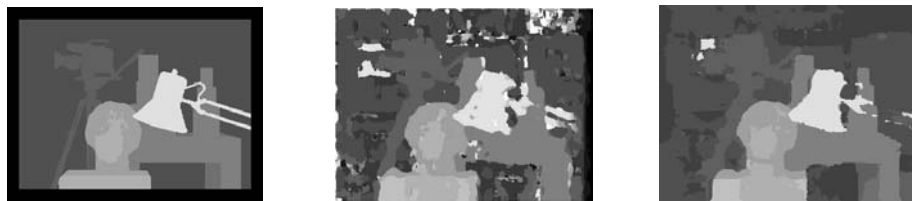
Fig.5 (a) ground truth of "Tsukuba" (b) the result with fixed windows (c) result of the algorithm
