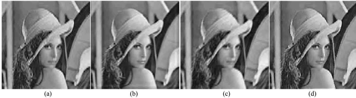
Fig. 1 The result: (a) Compressed image at 0.07 bpp; (b) Filtering method used in [7]; (c) Aria Nosratinia's method in [6]; (d) the proposed method in this article
