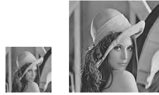
Fig. 6. Progressive access. The left image is decrypted with the key for resolution 3, and the right one is decrypted with the key for resolution 4. However, it is impossible to obtain the right image using the key for resolution 3.
