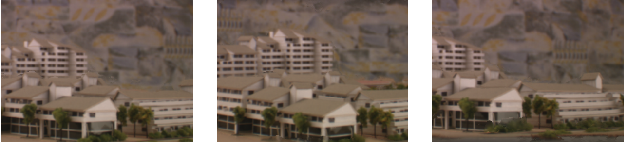
Fig. 5. All in-focus images are generated for arbitrary viewpoints using the proposed focus measure.
