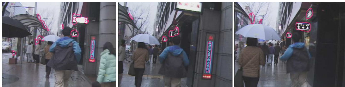
Fig. 4. Result example for a movie image stream. Pink curves indicate extracted character / text regions.
