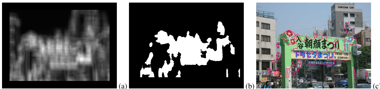
Fig. 2. Result example: (a)likelihood image A_H , (b)B/W image obtained by a threshold process, (c)extracted character / text regions (surrounded by pink curves) superimposed on the original image.
