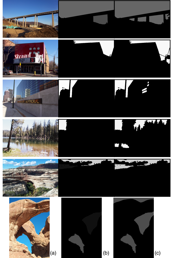
Figure 6. Algorithm results. (a) Original images. (b) Initial sky belief maps. (c) Final belief maps from the algorithm.
