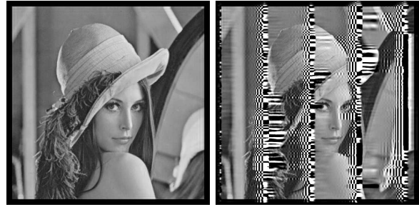
Fig. 4. Reconstructed images with tree-structured OFB: with no erasure (left), Burst of 31 erasures starting with the lowpass component (right).
