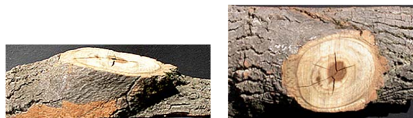
Figure 3 — Side and top views of a sound knot defect.
