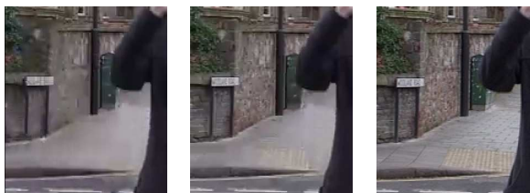
FIGURE-6 : Detail of decoded frame with a short term IDR frame (left) and a long term IDR (middle). The original frame is also shown (right).
