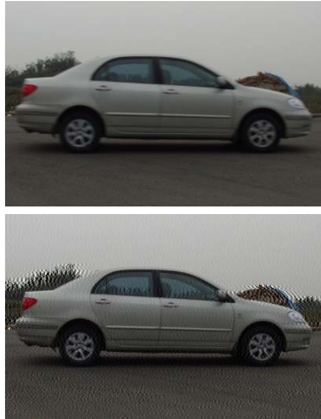
Fig. 2. Vehicle speed detection with known speed: (top) the original motion blurred image, (bottom) the restored image.
