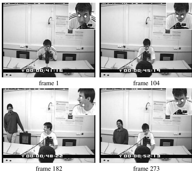
Fig. 3. A few frames of the sequence used in Experiment I, with the tracking results of the two individual trackers imposed (marked by dots). After the head rotates to the right, the right eye becomes occluded, causing an irrecoverable failure.
