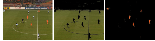
Fig. 2. Classification of color areas with grass ( 2.b) and players from one team ( 2.c) based on kernel density classification from ( 2.a).
