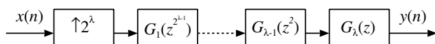
Fig. 1. A one-dimensional DWT synthesis filter bank. Signal x(n) in subband \lambda is transformed inversely to signal y(n) in the temporal domain.
