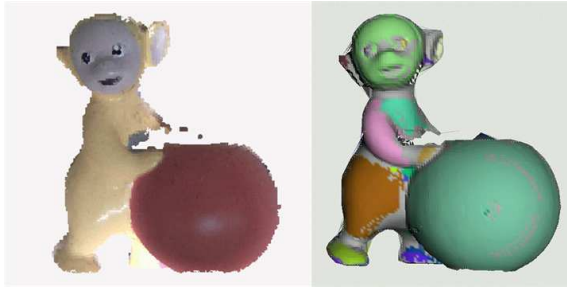
Fig. 3. Part decomposition - range image (left), decomposed parts represented by different colors (right) with \alpha = 0.1 , \beta_1 = 0.01 and \beta_2 = 0.01 .
