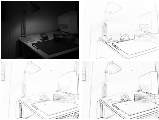
Fig. 2. Suppression of the illumination influence on the derivatives. Upper left: grey value image. Upper right: gradient |f_x| + |f_y| . Lower left: gradient of \ln f . Lower right: gradient of \ln(1 + f) with pre-processing. All gradient images were scaled to the maximum grey value.
