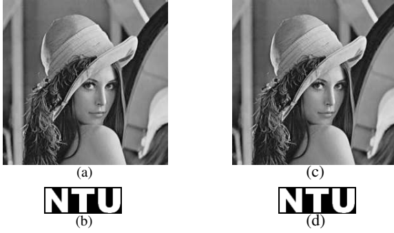
Fig. 4. (a) The original Lena image, (b) the grayscale watermark ('NTU' is the abbreviation of 'Nanyang Technological University'), (c) the watermarked Lena image and (d) the extracted watermark.
