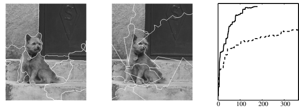
Fig. 2. Data driven vs. random proposals. Left : result of data driven segmentation after 179 samples. Center : result of segmentation using random proposal distributions in the same amount of CPU time (365 samples). Metropolis-Hastings acceptance probabilities were 27 % and 20 %, respectively. Right : evolution of log posterior probabilities \log p(\mathbf{S}|I, M) in the MCMC chains with data driven ( continuous ) and random ( dashed ) proposal distributions.
