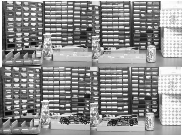
Figure 6. Results of inserting an artificial object into the real scene. First row: The first and the last image of the laboratory sequence. Second row: A synthetic car, which is drawn by wire-frames, was inserted into the real scene. Demonstration video can be found at http://www.cse.cuhk.edu.hk/~khwong/demo/
