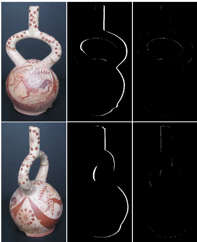
Fig. 4. Geometry enhancement for a Moche vase. Left: two frames of the original sequence; middle: contour error after camera calibration; right: contour error after proposed optimization.
