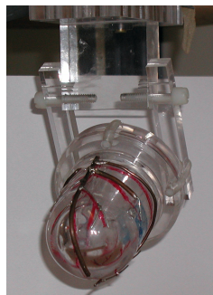
Fig. 3: Heart phantom. It is a structure made of PMMA (Poly Methyl MethAcrylate) which approximates the shape of a heart thanks to a cylinder having a half-sphere put on it. Such two cylinders form a double hull in which a radioactive tracer can be introduced for simulating the examination of tomoscintigraphy. A metallic tree, opaque to X-rays, is set onto the surface of the external cylinder and of the half-sphere to obtain the examination of coronarography.
