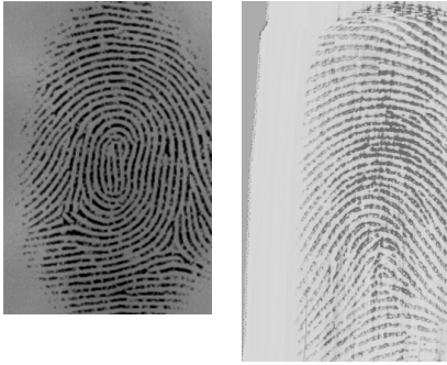
Figure 2: example of synthetic fingerprint (left, before decomposition) and sweep sensor image of real finger (right, reconstructed).
