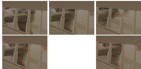
Fig. 1. Top row: Frames n - 1, n, n + 1 of a sequence showing PM; note legs and arms show heavy blur and are simply not well correlated between frames. Bottom row: motion compensated frames n - 1, n + 1 showing poor picture reproduction in the region of PM.
