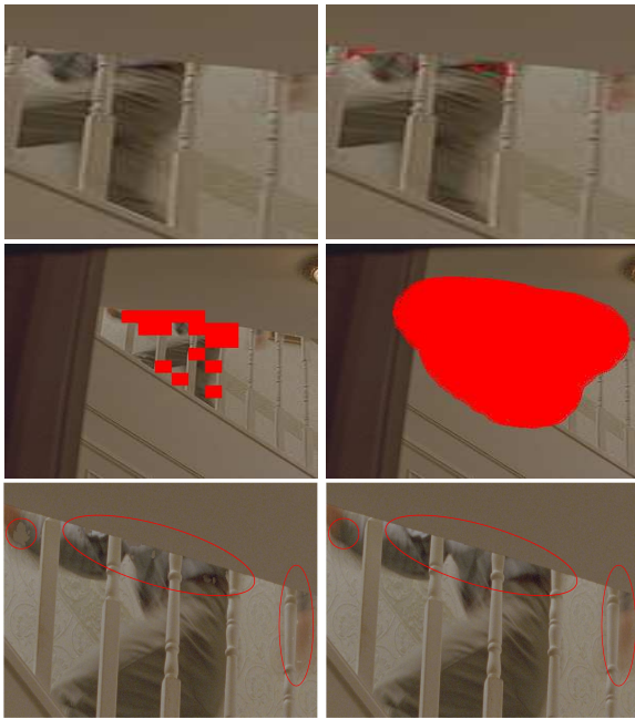
Fig. 2. Top row: Zoom on Original frame and detection using MRF model without PM detection. Middle row: Masks of PM (left [2]) and local motion (using the new technique presented) Bottom: Left degradation caused by dirt repair without regard to PM detection, right: dirt repair after PM detection .
