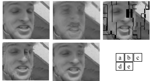
Fig. 3 Simulation results on the face portion of the Foreman frame 179. (a) Original frame; (b) Reconstructed frame using SMVF; (c) Predicted frame with interpolation errors; (d) Reconstructed frame using FR-MCI; (e) Reconstructed frame using IEC-MCI
