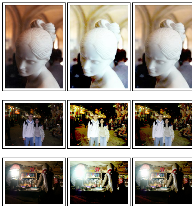
Fig. 2. Left-hand column: Underexposed input images; Second column: Lambertian-diffuse image recovered using our algorithm; Right-hand column: Output image (blending of the input image and the Lambertian-diffuse image).
