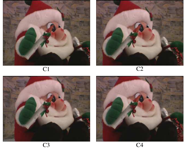
Fig. 3. The reference images (320 x 240 pixel) captured by 4 cameras located with interval of 20 [mm].
