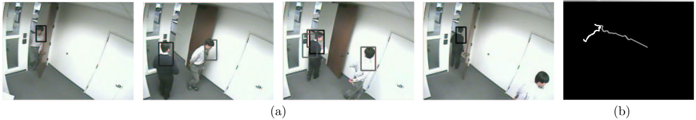
Figure 4: Tracking results of crossing tracks: (a) original images with overlaid bounding boxes showing the human detection results, (b) multiple object tracking result.
