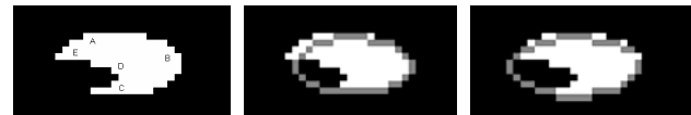
(a) Test image (b) With normal ellipse fitting (c) With precise ellipse fitting
