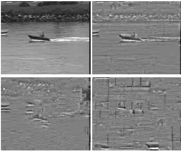
Fig. 1. Encryption results for Coast-guard . The encryption-approximation settings are: [top row, left to right] unencrypted, E1+A1 (PSNR 15.4 dB); [bottom row, left to right] E2+A2 (PSNR 16.2 dB), E4+A1 (PSNR 14.1 dB).
