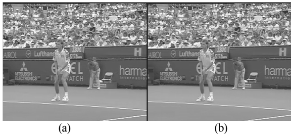
Figure 2. The Comparison of the 66 th frames of STEFAN with difference bit allocation techniques when QP = 22: (a) Constant quality (fixed QP) bit allocation (PSNR= 39.85 dB) and (b) Psychovisual model-based bit allocation (PSNR=34.19dB).
