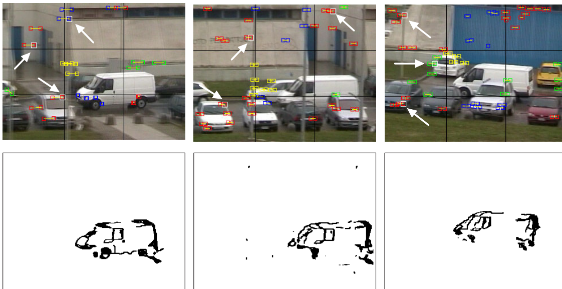
Fig. 2. Results of the feature clustering technique adopted to reduce the ego-motion effects. Top row shows the result of the tracking algorithm with highlighted, by the arrows, the features selected for the affine transform computation. Bottom row shows the results of the alignment process.
