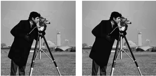
(a) Prune quadtree based denoising (SNR= 24.74 dB). (b) Prune-join quadtree based denoising (SNR= 24.73 dB).
