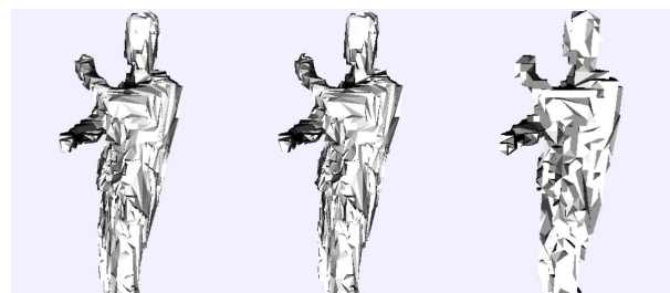
Fig. 4: Original mesh (left) and decoded meshes at 8 (middle) and 6 (right) bit per vertex
