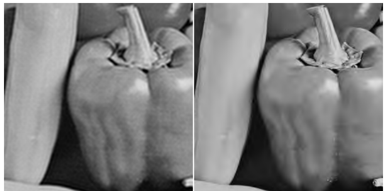
Fig. 6. Comparison of JPEG2000 and the proposed codec. Left: Proposed codec. Decimation rate 2x2, Bit rate 0.27bpp; Right: JPEG2000 Bit rate 0.27bpp
