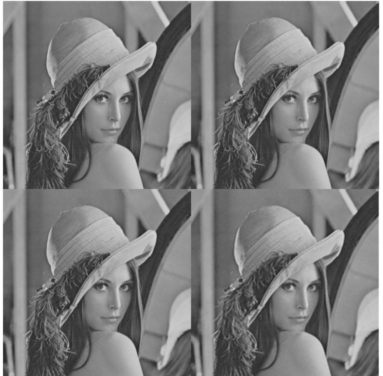
Fig. 4. Comparison of original and coded versions of “Lena”. Top Left: Original. Top Right: Decimation Rate 3/2x3/2 Bit Rate 0.97 bits/pixel. Bottom Left: Decimation Rate 2x2 Bit Rate 0.55 bits/pixel. Bottom Right: Decimation Rate 3x3 Bit Rate 0.25 bits/pixel.
