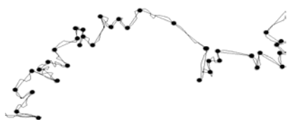
Figure 3. An example of reference lines obtained with polygonal approximation. The points of the reference line are marked with dots.
