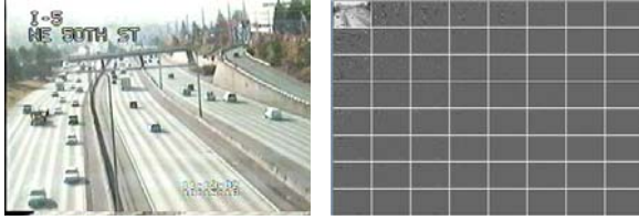
(a) A spatial frame (b) Image region matrix in DCT Figure 2 Comparison of spatial image and DCT image
