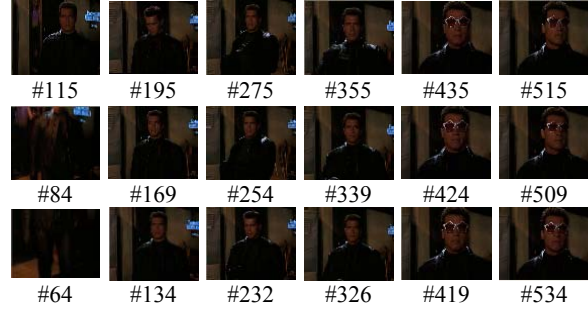
Fig. 6. Key-frames ( N = 6 ) selected form one shot of the “Terminator III” clip using the uniform (top-row), distortion-weighted (middle-row), and the proposed methods (bottom-row).
