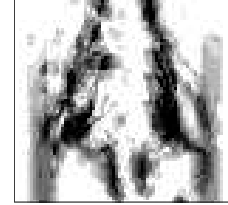
Fig. 3. The nose image representing the number of Left-Right inconsistent matching windows. The darker regions indicate that more matching window sizes are Left-Right inconsistent. The sloping region of the nose produces inconsistency for a greater range of matching window sizes.
