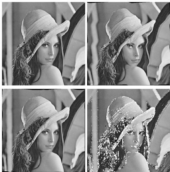
Fig. 1. Upper-left: original image; upper-right: artificially warped image; lower-left: reconstructed image; lower-right: original image showing in white color the points where a parametric model is detected.
