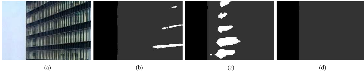
Fig. 3. Two-level texture map based on steerable filter decomposition. (a) Original grayscale image. (b) Texture classes at scale 0. (c) Texture classes at scale 1 (upsampled to original image size). (d) Combined texture classification.
