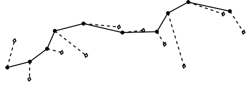
Fig. 4. A field of sensors (diamonds), along with the location of the tracked object at each time step (solid, circles), and the leader node measuring range at each time (dashed lines).
