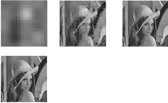
Fig. 16 Reconstructed images for 1, 3, 5 and 9 scans for the 4 Band wavelet transform and Modified EZW at Resolution 3.
