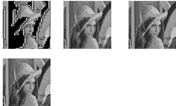
Fig. 15 Reconstructed images for 1, 3, 5 and 9 scans for 2-Band wavelet transform and Modified EZW at Resolution 3.
