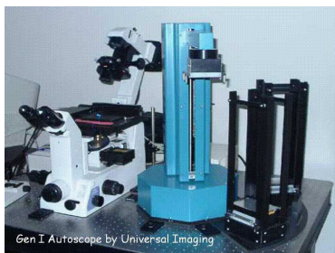
Figure 2: Gen I Autoscope: An automated fluorescence imager in the Institute of Chemistry and Cell Biology, Harvard Medical School [2].
