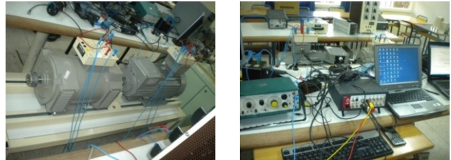
Figure 4. Wound rotor asynchronous motor & Data Acquisition System
