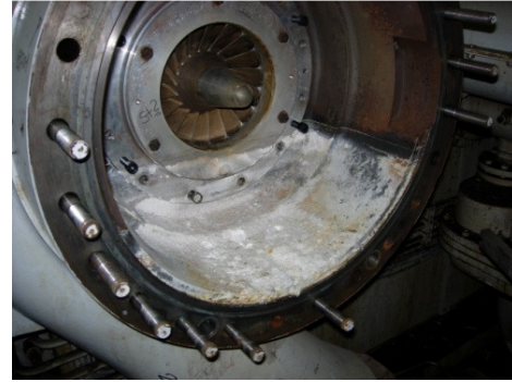
Fig.2. Fouling of a compressor stage: as it can be see, due to sea water leakage in the exchanger, sea salt can accumulate in the compressor frame.
